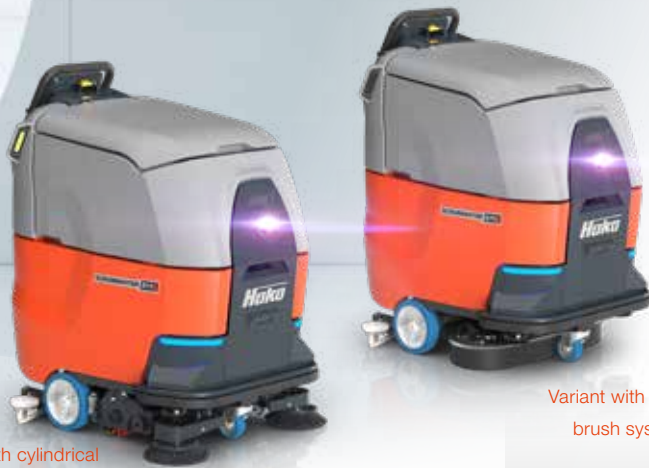
Variant with cylindrical brush system
